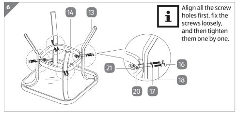
3. Attach the leg support 14 to the legs 13 with two M6 × 40 mm bolts 18, two washers 17 and two nuts 20 at each connection. Cover all bolts and nuts with bolt caps 16 and nut caps 21, respectively (see **Fig. 6**).
