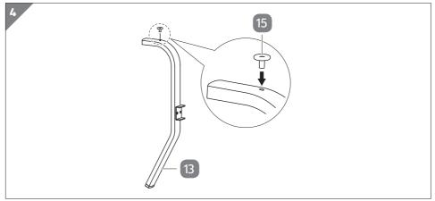
1. Attach a spacer **15** to the top of each leg **13** (see **Fig. 4**).
