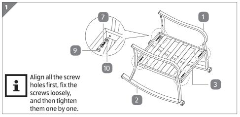
1. Attach the left armrest 1 and the right armrest 2 to the sitting surface 3 with one washer 10, one M6 × 25 bolt 7 and one bolt cap 9 at each connection (see **Fig. 1**).
