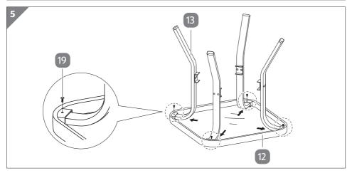
2. Insert the legs 13 into the brackets on the underside of the tabletop 12 and secure each leg to the tabletop with one M4 × 12 screw 19 (see **Fig. 5**).
