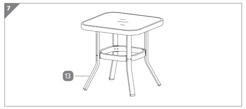
4. Turn the table over and place it on a flat and stable surface with all legs 13 touching the ground surface (see **Fig. 7**).
