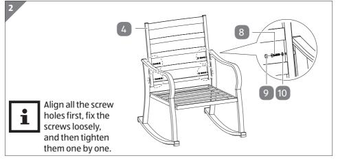
2. Attach the backrest 4 to the assembled structure with one washer 10, one M6 × 35 bolt 8 and one bolt cap 9 at each connection (see **Fig. 2**).
