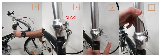
Make sure the quick release bolt snaps into the handlebar folding box (6). Then make sure the QR lever is tight before moving to the lock position. You may need a 10mm spanner to hold the nut whilst you turn the QR lever clockwise to tighten. If in any doubt call 01332 274242 (8).
