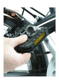
to unfold the pedals, pull and lift pedal step upward as in the images (12) (13)
