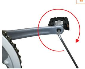
Kneel down at the right-hand side of the bike (the side with the chain) and present the left pedal (marked with an 'L' sticker) to the left hand crank.
