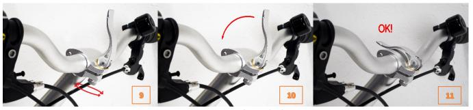
Tighten the quick release latch by pressing down the lever firmly (11)
