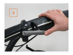
Tighten the stem with Allen key provided (4)
